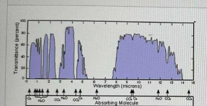
In the graphyou find the transmissivity of the atmosphere as a function of wavelength. In the table you find the bandwidth of the Meteosat Second Generation (MSG) satellite sensor.
